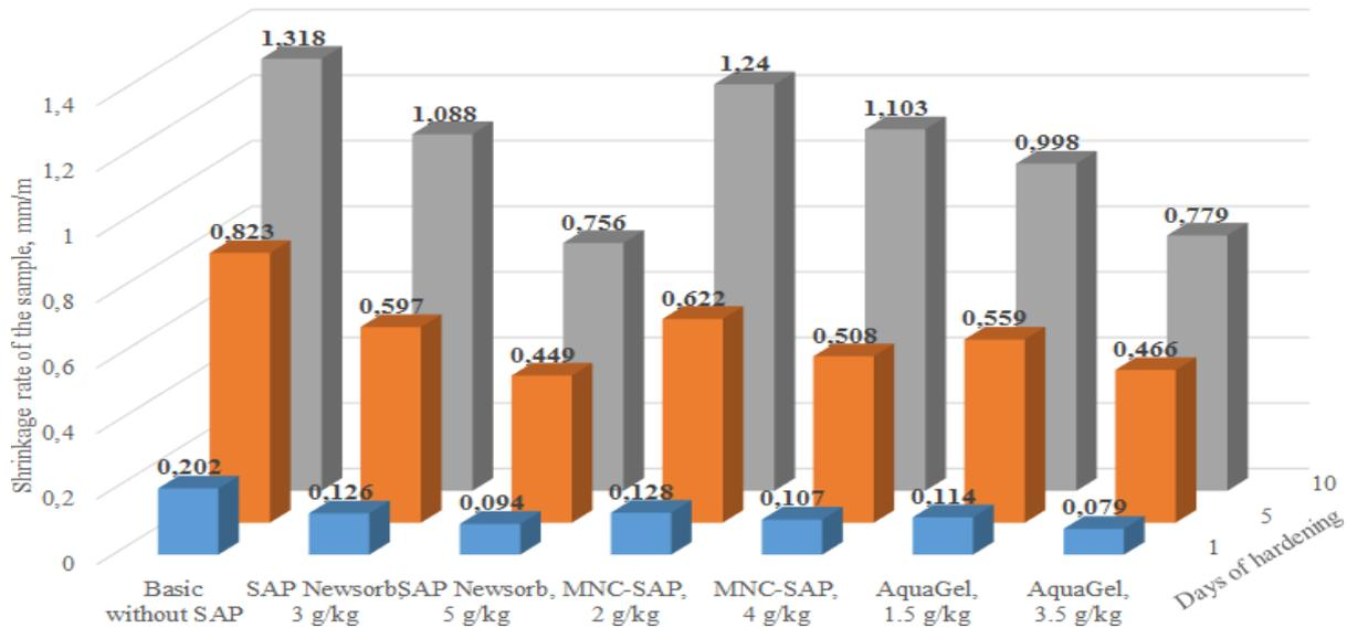
Fig. 1. Shrinkage rates on the 1<sup>st</sup>, 5<sup>th</sup>, and 10<sup>th</sup> days of samples' hardening
