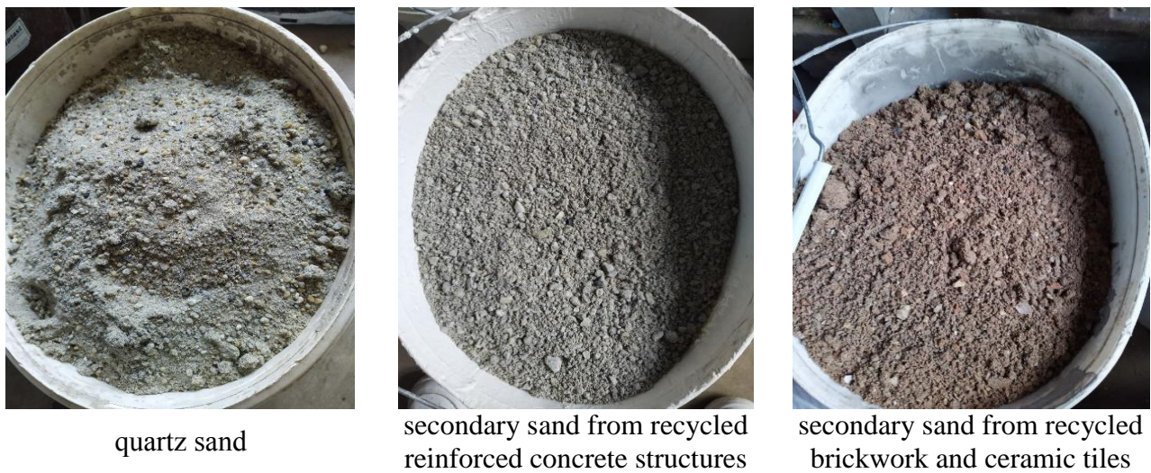
Fig. 2. Types of sand used for concrete production
