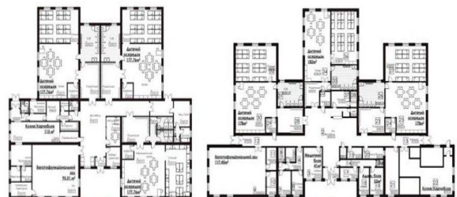
Fig. 3. The plan for a kindergarten with 45 to 60 places was developed by the Ministry of Regional Development
