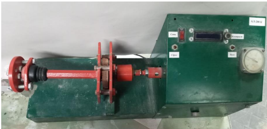
Fig. 1. Device for measuring adhesion by the tear-off method (top view)
