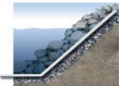
Fig. 2. Application of geotextile in hydraulic engineering
