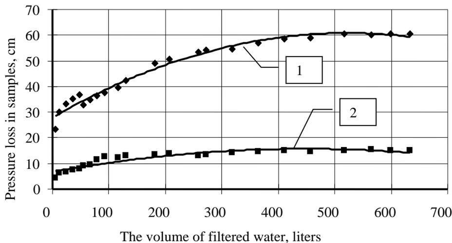
Fig. 7. Relationship between pressure losses and water volume:
