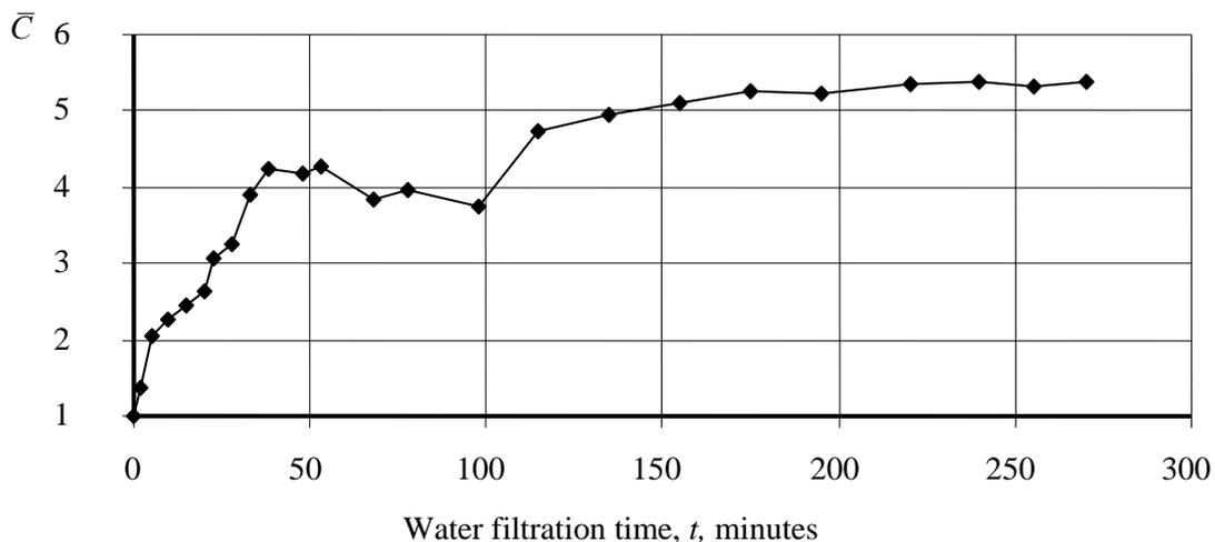
Fig. 5. Variation of polymer concrete resistance over time
