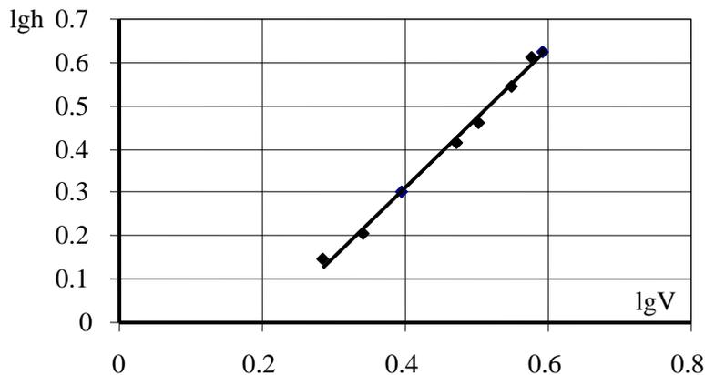
Fig. 3. Dependence of pressure loss on filtration rate in polymer concrete
