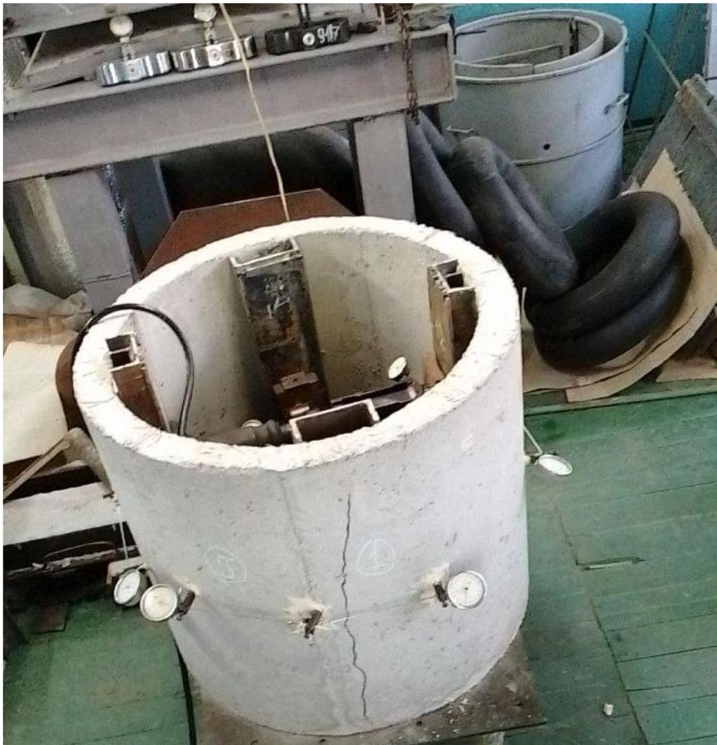
Fig. 1. Sample preparation: metal formwork and sample
