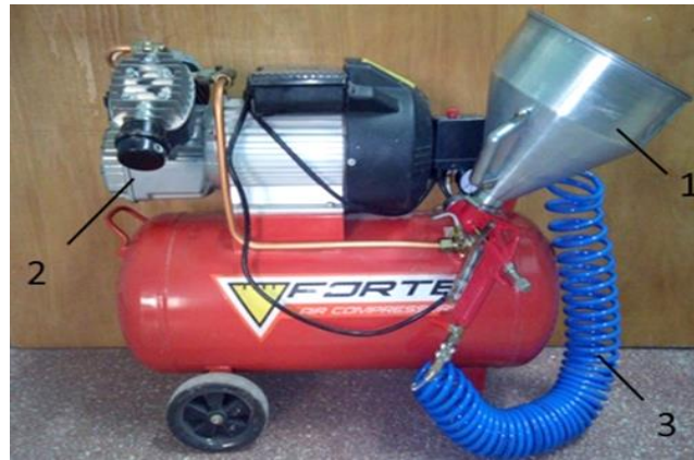
Fig. 1. Compact shotcrete installation: 1 – hopper; 2 – compressor; 3 – hose
