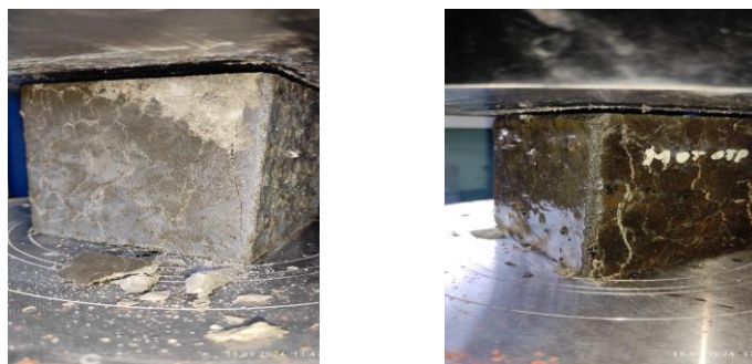
Fig. 3. Destruction on day 10 of a sample immersed in new 10W-40 motor oil
