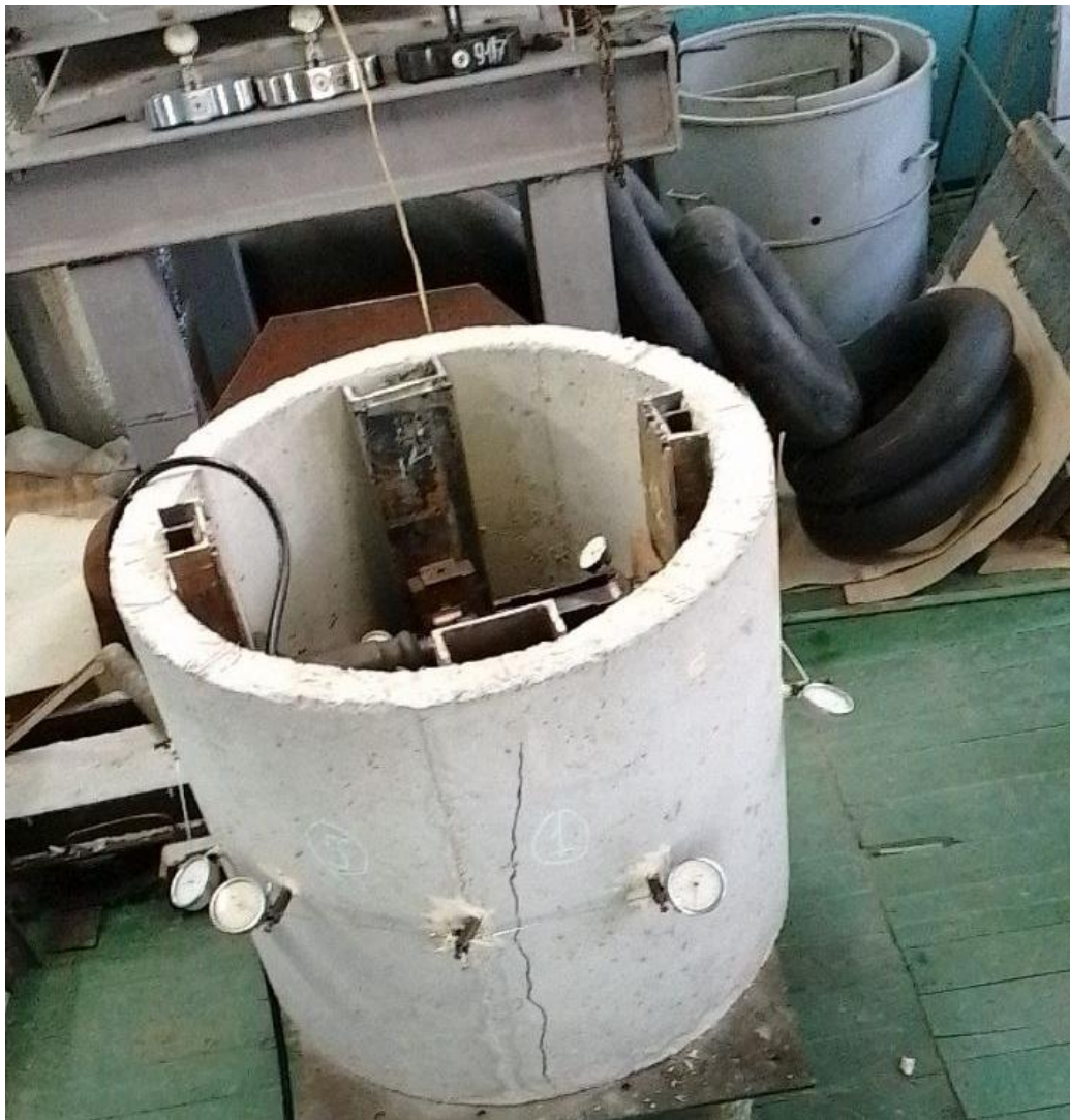
Fig. 1. Sample preparation: metal formwork and sample
