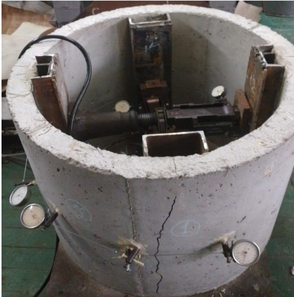
Fig. 2. Force platform for testing
