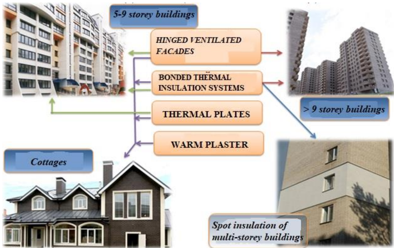
Fig. 1. Scheme of selection of thermal insulation systems for insulation and thermal modernization of facades
