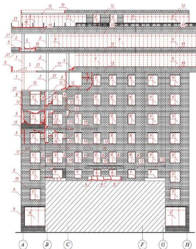
Fig. 5. Diagram of the location of the damage to the A-H facade
