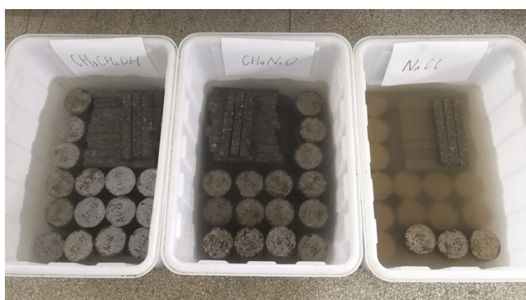
Fig. 1. The samples immersed in deicing salt solutions
