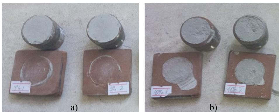
Fig. 3. Features of detachment of samples with different content of adhesive additive from the surface: a – 3%; b – 10%
