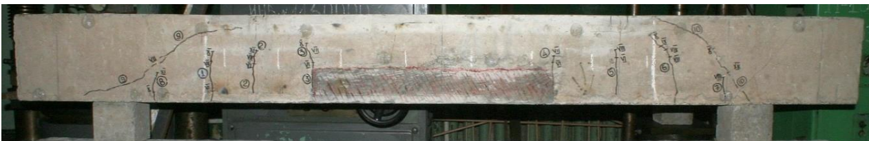
Fig. 4. Cracks in the sample RCD5
